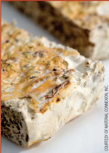
EcoCradle, a foamlike cushioning material from Ecovative Design, is an effective replacement for expanding polystyrene custom molded foams. Effectively the roots of mushrooms, the entire growing/creation process uses approximately 10 times less energy per unit of material than the manufacturing of synthetic foams, and the product is 100% biodegradable and compostable.
