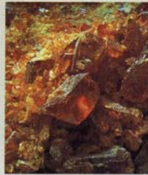
Natural linoleum is formed from a variety of rapidly renewable materials, including linseed oil, wood flour, and pine rosin (above left). During production, the ingredients are heated, mixed, and rolled flat (left). The sheets are cooled, backed with jute, then dried and trimmed. Pigments that do not contain heavy metals are used to achieve a wide variety of colors and unusual flooring installations (above right).
