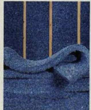
Cotton insulation (right) is produced with denim scraps from blue-jean manufacturing, diverting tons of material from landfills.
