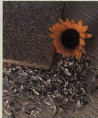
Wheatboard (far left) and sunflower board (left) mix agricultural "waste" with urethane-based binders to create an alternative to wood particle board.
