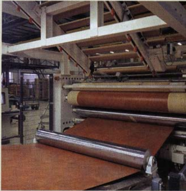
Natural linoleum is formed from a variety of rapidly renewable materials, including linseed oil, wood flour, and pine rosin (above left). During production, the ingredients are heated, mixed, and rolled flat (left). The sheets are cooled, backed with jute, then dried and trimmed. Pigments that do not contain heavy metals are used to achieve a wide variety of colors and unusual flooring installations (above right).
